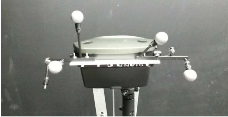
Figure 4.23 ST50 HMD with retro-reflective constellation
