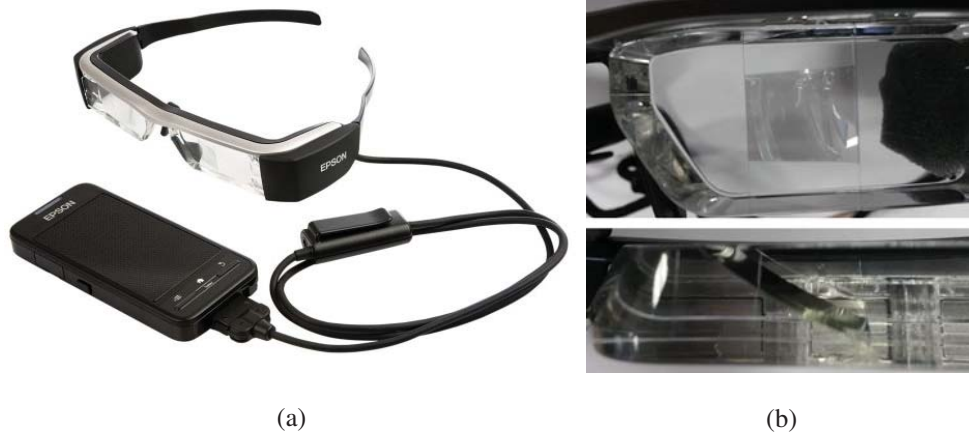
Figure 2.4 OST HMD with partially silvered mirror combiner
